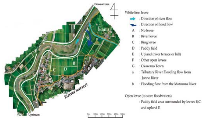
Concept of Open levee system
